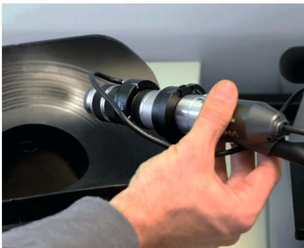
Visual quality control of the welding zone at the ELGEF Plus Branch Saddle Topload
